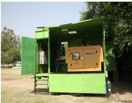
The Pyroformer™ is housed in a container unit that can be transported between villages and will be operated by the villagers themselves.
