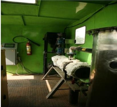
The Pyroformer™ converts waste products and residues (e.g., husk and straw) into oils, gas and biochar.
